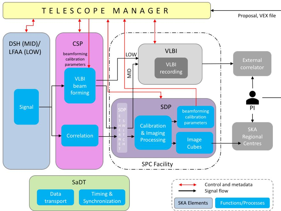
Figure 1. SKA-VLBI Capability for the SKA1 Observatory
